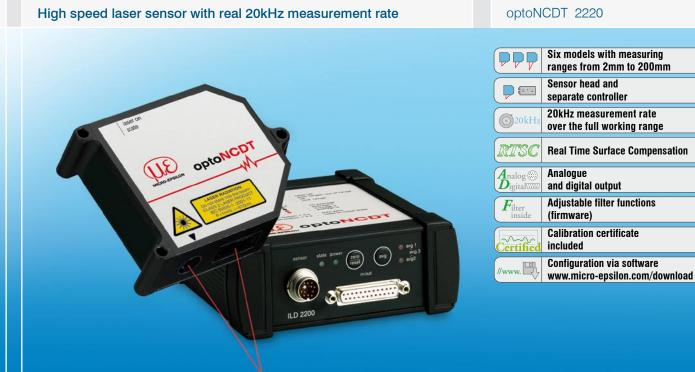
The optoNCDT 2220 provides a genuine 20kHz measurement rate for every measurement task. The series is ideally suited to superfast, complex applications and offers a high speed measurement with excellent resolution. In addition, the optoNCDT 2220 incorporates all the popular Micro-Epsilon benefits including the RTSC function for changing surfaces or the specific CCD-line for high resolution measurements.
