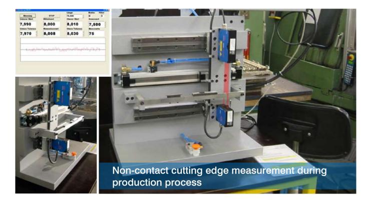
Cutting discs for the metal working industry are amongst the most common wear parts. In modern production, turned parts are manufactured to sub-micrometer precision. In order to ensure the accuracy of the machine tool requested, precise positioning of the tool is necessary, including the cutting discs.
