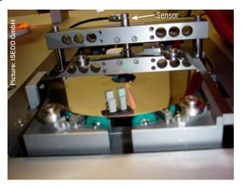
The measurement results are displayed graphically as a thickness profile across the measured circumference, the measured segments or other defined measuring processes. The evaluation contains the maximum and minimum thickness, the average thickness, the standard deviation and degree of variation.
