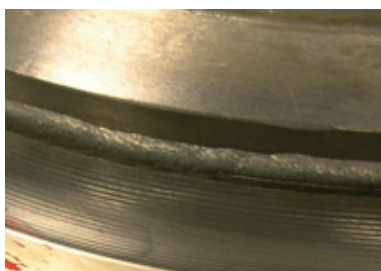
Welded seam OK
