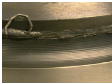
NOK: defect welded seam (flat profile and welding wire residues)
